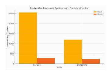
This graph contrasts ( $CO_2$ ) pollution from diesel and electric buses on two primary routes. Red Line Diesel buses emit 25,514 kg/day of CO<sub>2</sub>. Electric buses emit just 2,775 kg/day. Orange Line Diesel buses emit 11,948 kg/day. Electric buses emit only 2,275 kg/day. Both routes indicate an enormous reduction in emissions when electric buses replace diesel. For instance, emissions on the Red Line decrease by nearly 90% when using electric.
